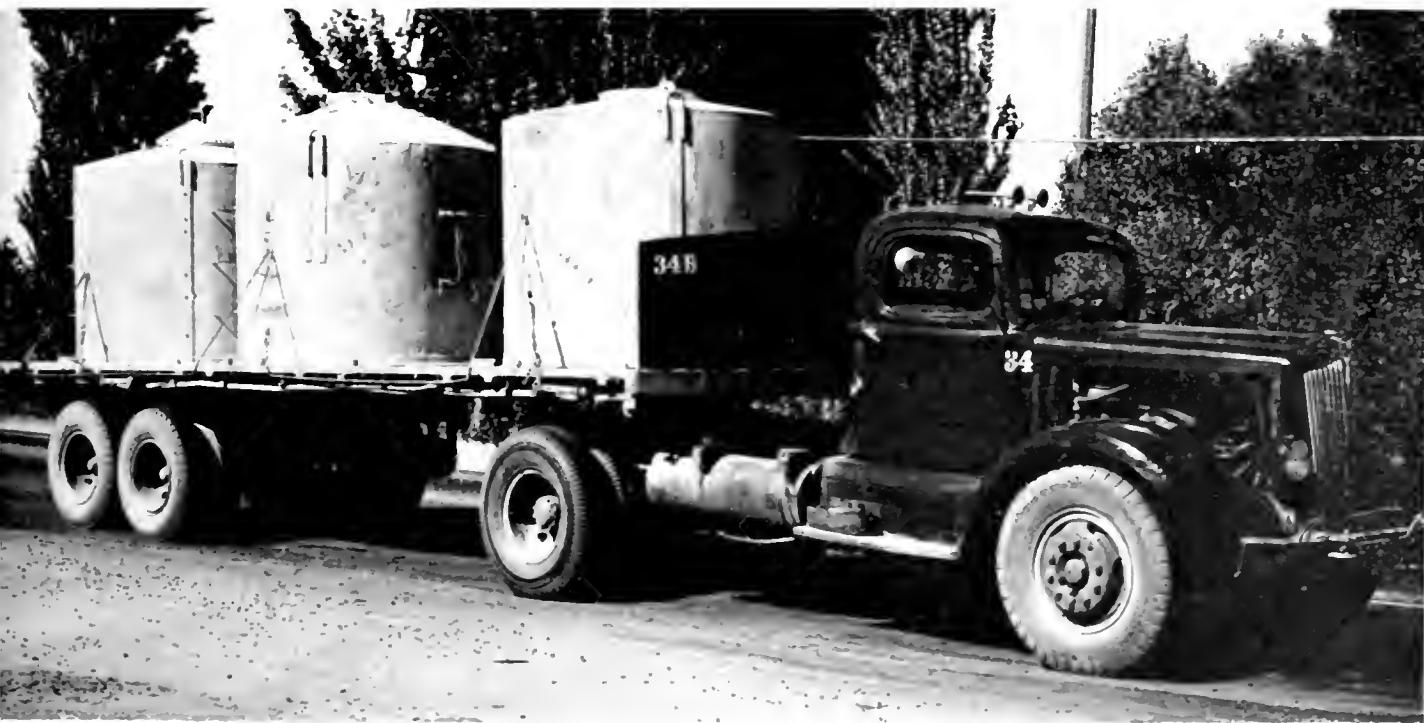
Thousands of tons of cement are being hauled by truck in large metal tanks as shown above
